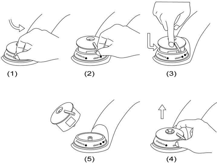
3. Turn the lid over and place on a table top. Pull out the anti-locking case. Using a brush or toothpick, check and remove any food or foreign particles that may be lodged in the floating valve. Replace the anti-locking case by pressing down.
