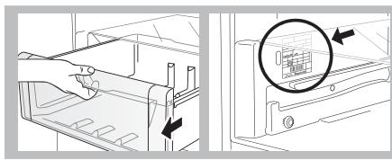
Let the refrigerator sit in an upright position for at least 2 hours before plugging it in. Check the information on the rating plate (110-120V with ground wire) (1.3.1, 1.3.2).
